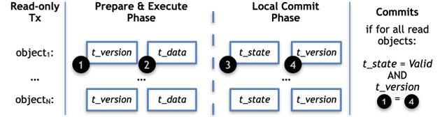
**Figure 6.** Zeus' consistent read-only transactions on readers.
