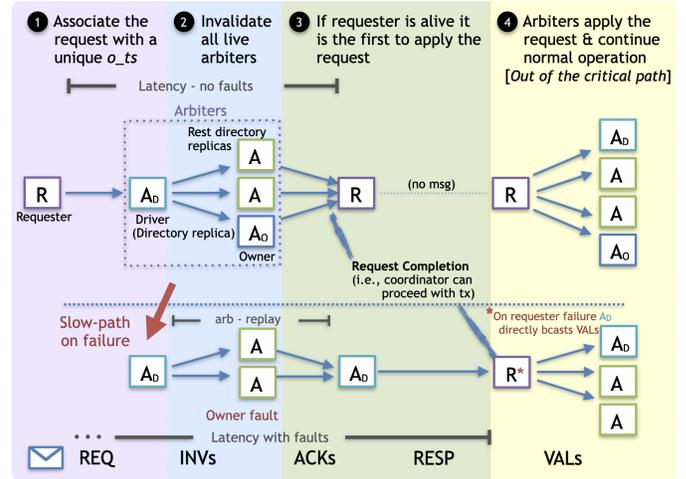
**Figure 3.** Zeus' ownership protocol with and without faults.
