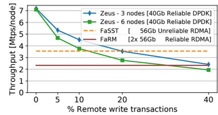
**Figure 9.** TATP while varying remote write transactions.
