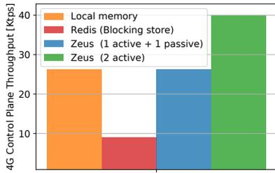
**Figure 13.** Cellular packet gateway control plane performance.
