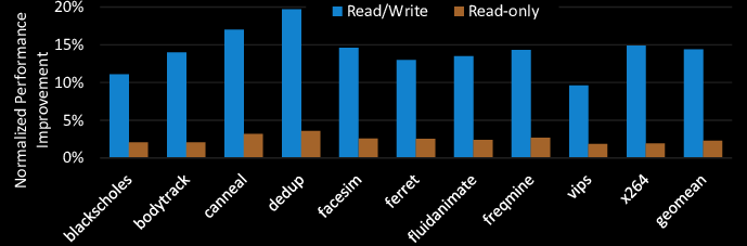
Figure 5. Performance improvement in a NG-LLC after eliminating remote access latency for read/write shared data.
